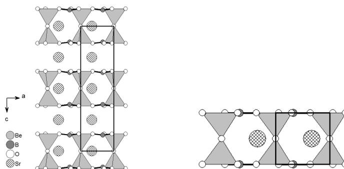
Figure 2. Side view of disordered SBBO structure showing elongated disordered unit cell (left) and new polymorph of ordered SBBO highlighting compact ordered unit cell.
