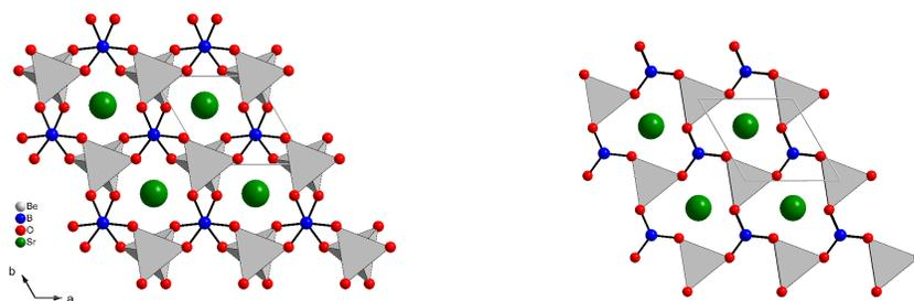
Figure 1. Top view of disordered SBBO structure showing rotated borate groups (left) and new polymorph of ordered SBBO highlighting perfectly aligned borate groups
